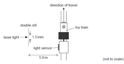
Light from a laser is incident on a double slit. The light from the slits is detected by a light sensor attached to the train.
