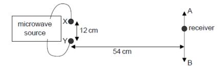
Maxima and minima of intensity are detected at several points along AB.
