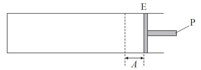
The piston P is displaced a small distance A from E and released. As a result, P executes simple harmonic motion (SHM). Define simple harmonic motion as applied to P.
