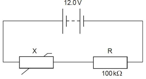
The battery has an electromotive force (emf) of 12.0 V and negligible internal resistance.
