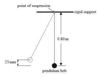
The point of suspension of a pendulum bob is moved from side to side with a small amplitude and at a variable driving frequency f.
