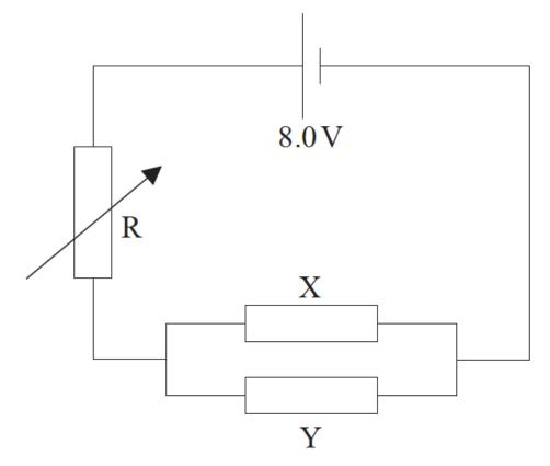
The resistance of R is adjusted until the currents in X and Y are equal.
