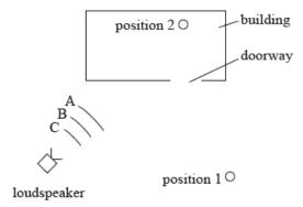
A, B and C are wavefronts emitted by the loudspeaker.
