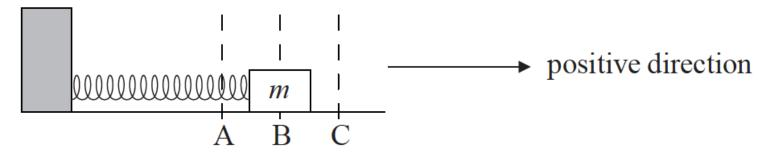
The equilibrium position is at B. The direction B to C is taken to be positive. The object is released from position A and executes simple harmonic motion between positions A and C.
