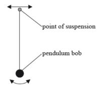
For each value of the driving frequency a steady constant amplitude A is reached. The oscillations of the pendulum bob are lightly damped.
