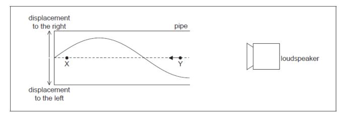
X and Y represent the equilibrium positions of two air molecules in the pipe. The arrow represents the velocity of the molecule at Y.
